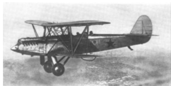
The towplane R-5 was a powerful multipurpose airplane from Polikarpov. Max climb of the R-5: 6 m/s
